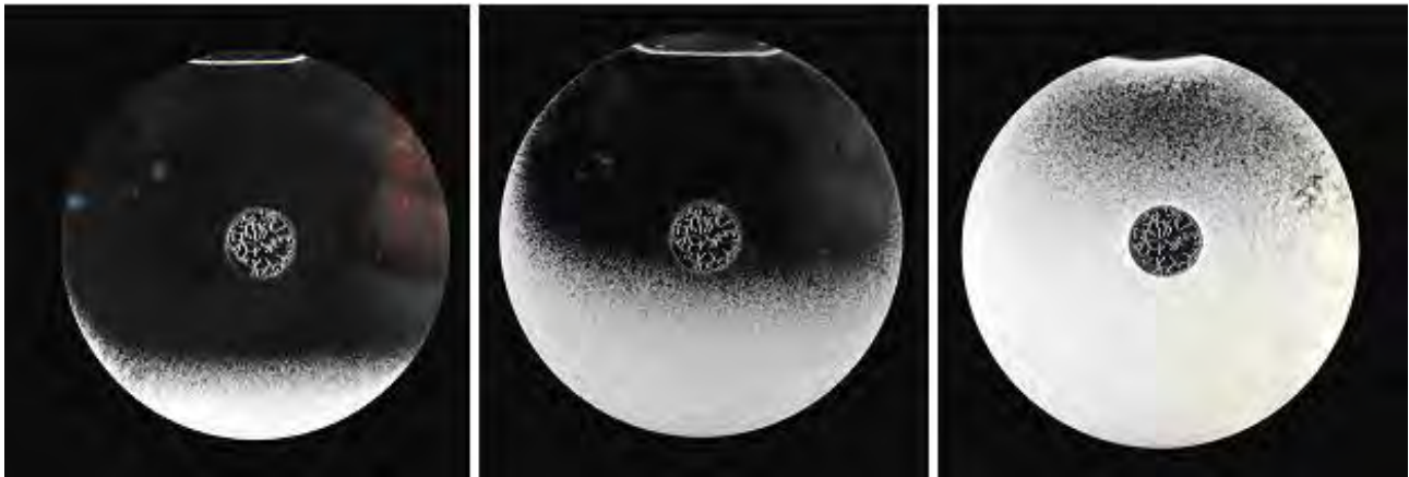
Figure 2. Prototype 1, 2.5mm interlayer, Organic PCM, Specific Heat 197 kJ/kg, Melting Point 29 °C, 6-minute transition
