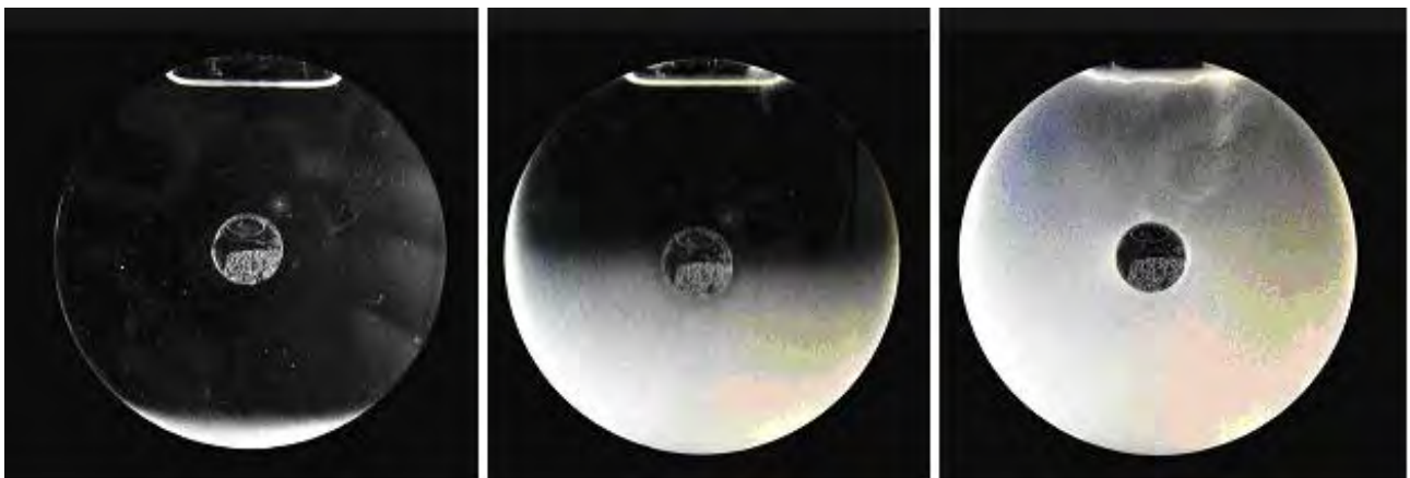
Figure 3. Prototype 2, 5mm interlayer, Organic PCM, Specific Heat 197 kJ/kg, Melting Point 29 °C, 9-minute transition
