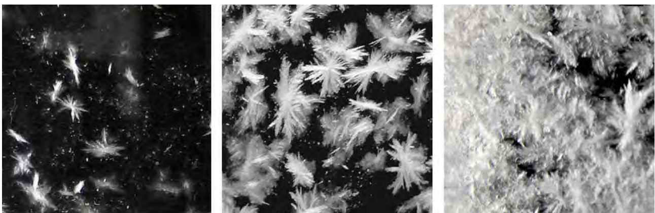
Figure 6. Prototype 4, Time-lapse close-up dendrite crystallization
