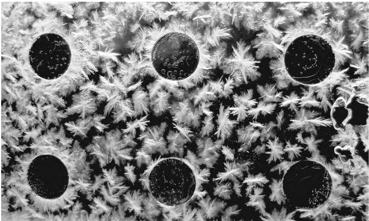
Figure 5. Prototype 4, 2.5mm interlayer, Organic PCM, Specific Heat 197 kJ/kg, Melting Point 29 °C
