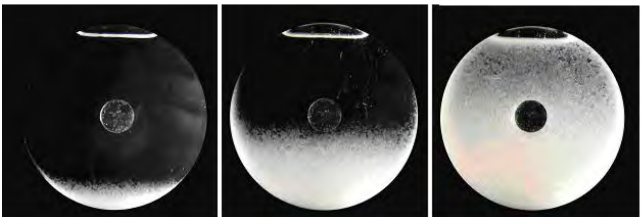
Figure 4. Prototype 3, 7.5mm interlayer, Organic PCM, Specific Heat 197 kJ/kg, Melting Point 29 °C, 15-minute transition
